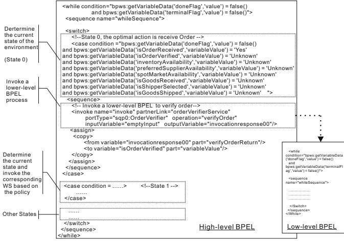
Fig. 5. A snippet of the WS-BPEL flow for the supply chain process. The verifyOrder operation is an abstract action whose invocation leads to the execution of a lower level Web process.
